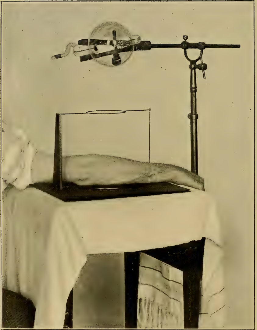
PLATE 50.—Author's Distortion Landmark. Method of use. This Instruction Plate shows the tube centred at twenty inches over the photographic plate on the base of the Author's Position Finder, as taught in the text. In the radiograph that will result from this exposure the negative will contain medico-legal proof of the position and distance of the tube, the field of the axis of the rays, and the degree of "distortion" present, if any has been caused. See frontispiece for example of radiographic evidence thus obtained.
